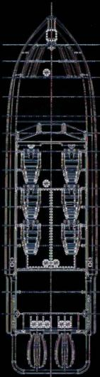
Overall Length 9.20 m 2.65 m Beam 8.78 m Waterline Length 1.34 m Depth 0.45 m Draft 4800 kg Displacement 2x300 HP Outboard Engine 45 knots Maximum Speed 28 knots Cruise Speed Total 530 lt Fuel Tank 330 Nm Range@Cruise Speed Range@Maximum Speed 220 Nm Aluminum 5083 H321-AIMg4,5 Material
